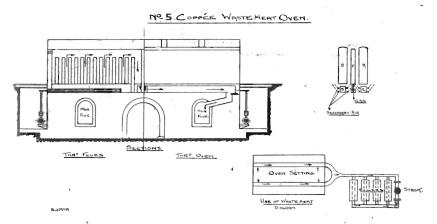
The gases for heating the oven walls are brought back from the by-product plant in the two gas mains, shown either end of the oven, led through a mixing chamber fixed on smaller tube, similar to the Bunsen burner, then into the fireelay tubes running under the uptakes, corresponding to each flue an aperture is drilled, naturally of varying diameters. Running parallel with the sole flues "S and S," will be noticed secondary air openings; combustion taking place at the base of each uptake, the
