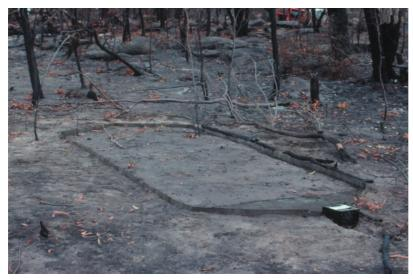
Fig 3. Plot 1, a 9 m<sup>2</sup> closed plot installed on a crest to measure soil loss in t ha-1
