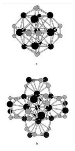
FIGURE 13. The optimised structures of the copper carbohedrenes (a)  $[Cu_{13}C_{12}]^+$ , (b)  $[Cu_{25}C_{24}]^+$ .
