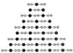
FIGURE 14. The structures of the gaseous metal cyanide Ions  $[Cu_{X}(CN)_{X-1}]^{+}$  and  $[Cu_{X}(CN)_{X+1}]^{-}$ . Cu atoms are dark, C atoms grey, N atoms hatched.
