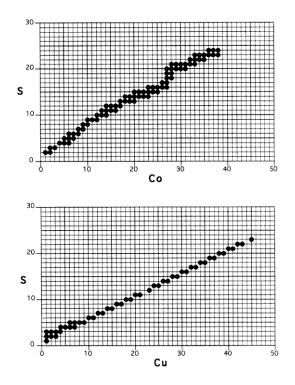
FIGURE 9. Maps of the compositions of the ions  $[Co_xS_y]^$ generated by laser ablation of CoS, and of the  $[Cu_xS_y]^-$  ions formed by laser ablation of various copper solid solids.
