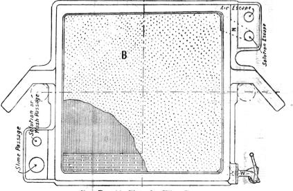
FIG B.-Air Plate for Filter-Press.
