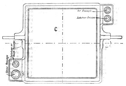
FIG. C.-Open Plate or Slimes Plate for Filter-Press.
