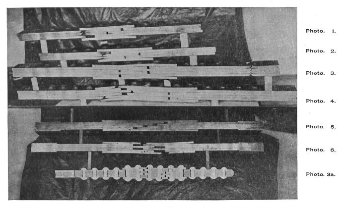
PHOTOGRAPHS OF THE SPECIMENS OF RIVETED JOINTS TAKEN AFTER THEY WERE TESTED.
