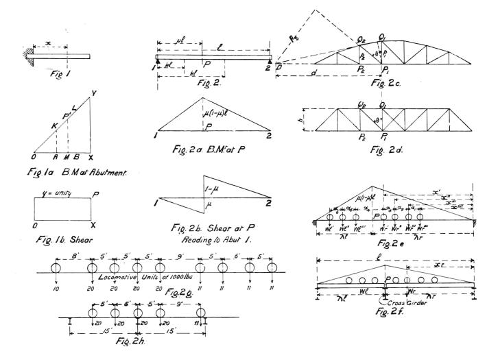
Assume B. Mt. as positive when in same direction as the B. Mt. caused by the reactions at the abutment.
