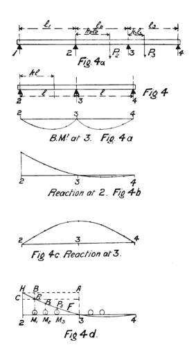
The girders are assumed continuous over three supports on the same level; and the equations as deduced below are got from the equation of three moments, proofs of which are given in many text-books.  $\dagger$
