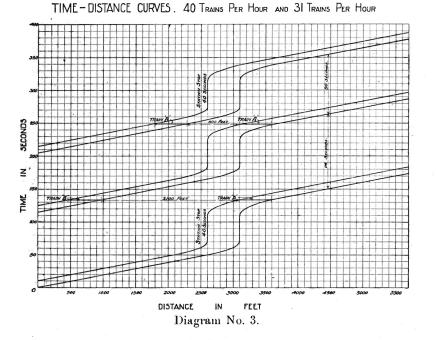
During constant speed running the distance time graph is two parallel straight lines, the tangent of their inclination to the ordinates being a measure of the speed. During uniform deceleration the graph becomes two parabolas, concave upwards; during a stop (at a station for example), the lines again become parallel but vertical, and during acceleration, if uniform, they again become parabolic but convex upwards.
