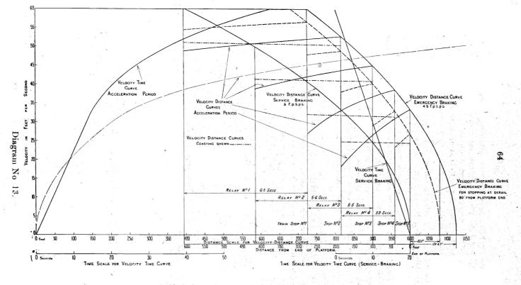
DIAGRAM Shewing Arrangement of Relays and Train Stops necessary to stop within 124-4 FT bevond Platform or to derail at 80 FT bevond Station wit 13-6 MRH Max. Speed.
