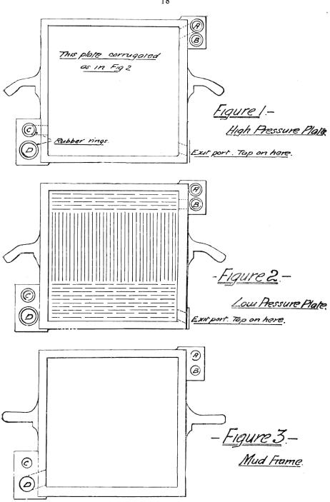
The press is fitted with four channels (see figures 1, 2, 3, and 4)—there may be more for special purposes; a, is to allow the air to escape from the press and communicates only with every alternate solid or 'High Pressure' plate; b, is the wash solution exit channel and communicates with 'the other solid or 'low pressure' plate; c, is the wash entrance channel, and communicates with the high pressure plates; d, is the sludge channel, and communicates with the hollow frames only.
