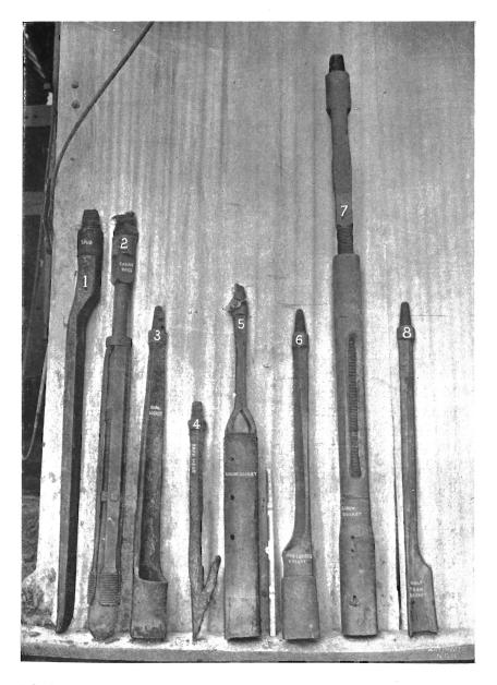
Spud. 2. Casing Dogs. 3. Oval Socket. 4. Rope Hook. 5. Casing Socket. 6. Socket. 7. Screw Socket. 8. Half-turn Socket.
