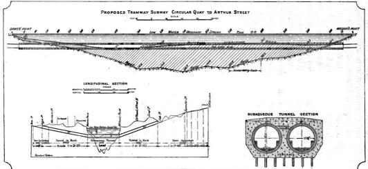
Note.—Datum for Borings, Low Water Ord. Spring Tides. Datum for Tunnel (Standard) Mean Sea Level, 2.52 above Low Water.
