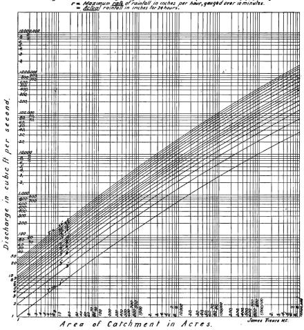
Nº2 Discharges by Formula Nº3 Q=(+78+ orr±-ozlogA)logA+ logr. r = Maximum rate of rainfall in inches per hour, gauged over io minutes. = Actual rainfall in inches tor zehours. Diagram
