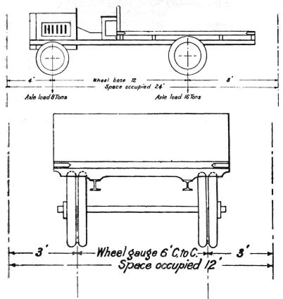
For closely packed heavy vehicular traffic a distributed load of 100lbs. per square foot may obtain over the whole bridge. It is not considered possible that it can be exceeded. The average heavy traffic will be very much less. The high figure was adopted so that no restriction or regulation of the roadway traffic will ever be needed.
