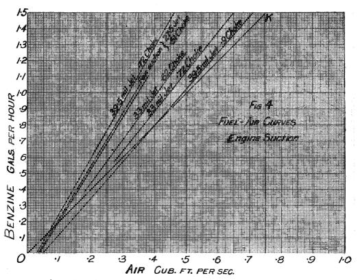
since A and a remain constant for any one curve. That is, the fuel is directly proportional to the air, and the relation is represented by a straight line curve.
