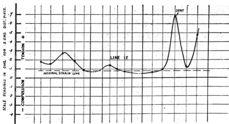
FIG. 11.—Curve of longitudinal strains obtained along line 2.
