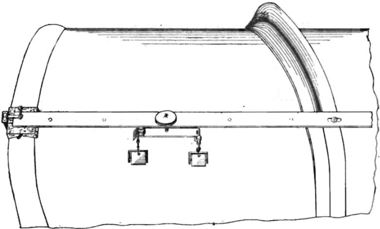
FIG. 9.—Diagram showing method of applying Martens' Extensometer.
