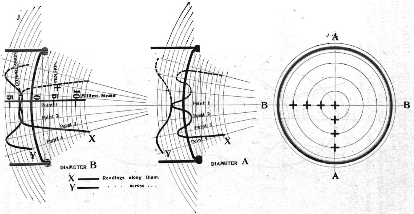
FIG. 15.—Curves of strain on dished ends. The fourteen short black lines on the right-hand diagram show the positions of the distance pieces for the respective series of observations.
