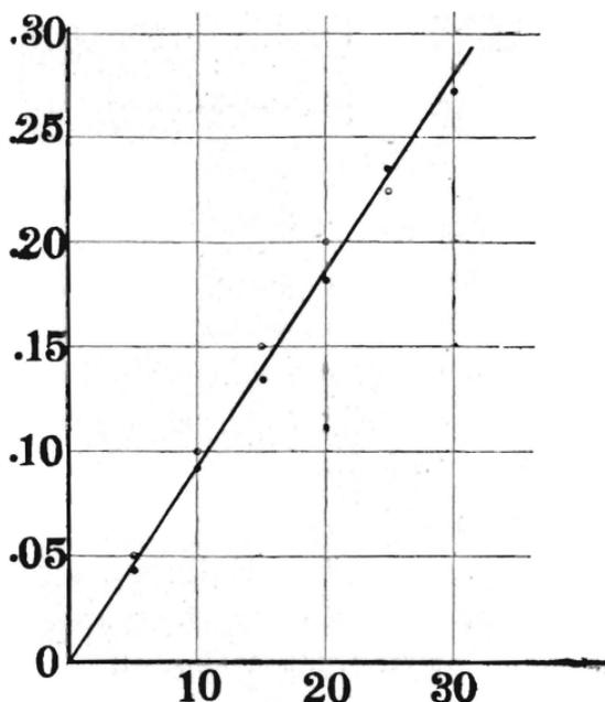
FIG. 10.—A typical curve showing strains (scale readings, cms.) produced by pressure in drum up to 30 lbs. per square inch. Dots show ascending readings and circles descending readings.
