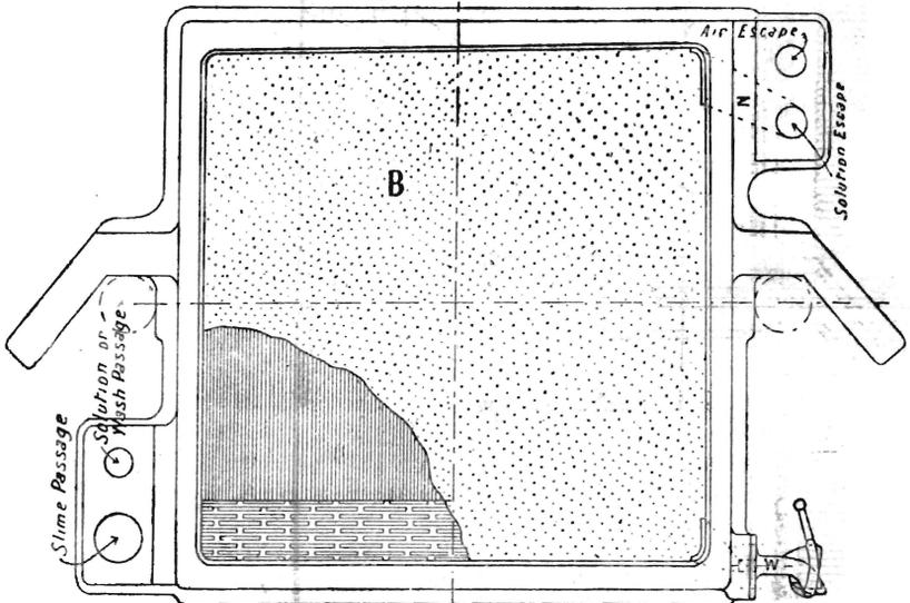
FIG. B.—Air Plate for Filter-Press.
